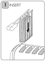
Set 'selector' and starting from the left insert cage into the slots. Push down until clamped tightly shut.
